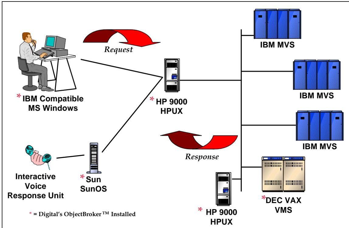
Figure 5 - Simplified System Diagram of the CRS application<sup>2</sup>.
